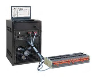
The EVd-40 can discharge batteries at high power (10,000 watts). A Prius battery subjected to this discharge power will exceed initial currents of 40 amps.
